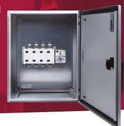
400A 4 pole manual changeover switch in a metal enclosure to IP65. Enclosure has separate lock. The switch handle is padlockable and defeatable. Earth studs are fitted and fixing brackets and earth straps are included
