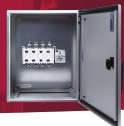
630A 4 pole manual changeover switch in a metal enclosure to IP65. Enclosure has separate lock. The switch handle is padlockable and defeatable. Earth studs are fitted and fixing brackets and earth straps are included
