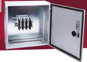
800A 3 pole switch fuse in a metal enclosure to IP66. Enclosure has separate lock and reversible door for gland plate either top or bottom. The switch handle is padlockable and defeatable. The switch fuse accepts BS88 fuse links. All terminals are provided with shrouds. Earth studs are fitted and fixing brackets and earth straps are included
