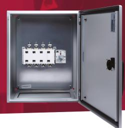
800A 4 pole manual changeover switch in a metal enclosure to IP65. Enclosure has separate lock. The switch handle is padlockable and defeatable. Earth studs are fitted and fixing brackets and earth straps are included
