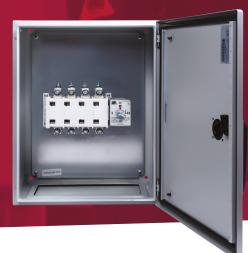
800A 4 pole manual changeover switch in a metal enclosure to IP65. Enclosure has separate lock. The switch handle is padlockable and defeatable. Earth studs are fitted and fixing brackets and earth straps are included
