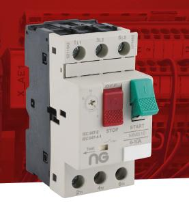
Manual motor starters combine motor control with protection against short circuit, overload and phase failure. Auxilliary contacts are front mount, snap fit. The operating handle is lockable in the OFF position. Large scale dial has lockable flap.
