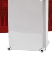
Glass fibre reinforced polycarbonate adaptable box for use in harsh environments. Opaque lid fixed with four screws. Moulded base has various fixing points for backplates and printed circuit boards.
