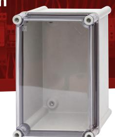
Glass fibre reinforced polycarbonate adaptable box for use in harsh environments. Transparent lid fixed with four screws. Moulded base has various fixing points for backplates and printed circuit boards.
