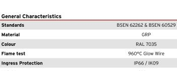
**Ingress Protection** Height 270mm Width 180mm Depth 141mm -30°C to +60°C **Operating Temperature** Weight 1.18 Kg
