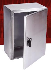
Wall mounting stainless steel enclosure with brushed finish. The polyurethane gasket keeps its profile over time to give a high degree of protection against water and dust. Door opens 125° and is reversible. Welded earth studs top and bottom. Fitted, galvanised backplate has return edges for extra rigidity
