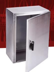
Wall mounting stainless steel enclosure with brushed finish. The polyurethane gasket keeps its profile over time to give a high degree of protection against water and dust. Door opens 125° and is reversible. Welded earth studs top and bottom. Fitted, galvanised backplate has return edges for extra rigidity
