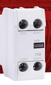
Auxiliary Contacts provide 16A AC1 additional signalling function, in combinations of normally open and normally closed contacts. Top mount devices clip onto concators; side mount are screw fixed
