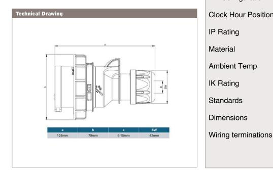
Technical Specifications Colour Red Rating 16A Voltage 400v (50/60Hz) Pin Configuration 4 pin (3P+E) Clock Hour Position 6h **IP** Rating **IP67** Material Polyamide 6 (PA6) -25°C ~ 40°C **Ambient Temp IK10 IK Rating** BS EN60309-1&2 Standards
