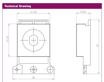
**Technical Specifications** Material Nylon Back Box Depth 35-47mm White Finish Supplied with Dimmer knob and fixing nut Frontplate Compatibility NSP622, NSP632, NSP642, NSP662 **Dimmer Compatibility** LEDDIM120 Modular Yes Warranty 20 Years **IP Rating** IP20 **Operational Temperature** -5° to +40°C Standards BS5733 Dimensions 52x40x13.5mm (HxWxD)
