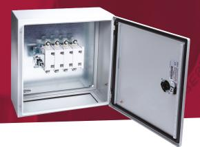
200A 4 pole switch disconnector in a metal enclosure to IP65. Enclosure has separate lock and reversible door for gland plate either top or bottom. The switch handle is padlockable and defeatable. All terminals are provided with shrouds. Earth studs are fitted and fixing brackets and earth straps are included
