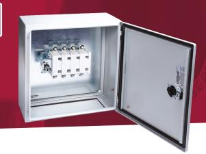
250A 4 pole switch disconnector in a glass reinforced polycarbonate enclosure to IP65 IK10. Enclosure has separate lock and reversible door. The switch handle is padlockable and defeatable. All terminals are provided with shrouds.
