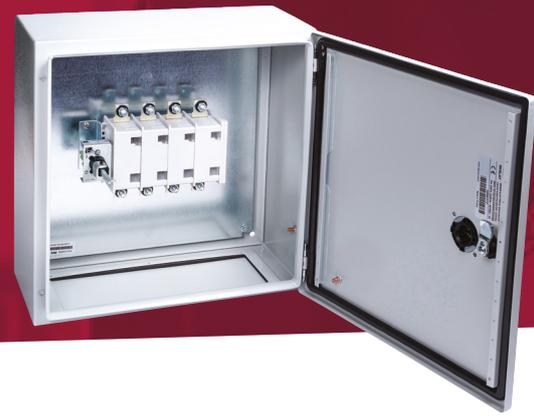
**315A 4 pole switch disconnecter in a metal enclosure to IP66. Enclosure has separate lock and reversible door for gland plate either top or bottom. The switch handle is padlockable and defeatable. All terminals are provided with shrouds. Earth studs are fitted and fixing brackets and earth straps are included**
