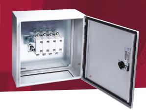
400A 4 pole switch disconnector in a metal enclosure to IP65. Enclosure has separate lock and reversible door for gland plate either top or bottom. The switch handle is padlockable and defeatable. All terminals are provided with shrouds. Earth studs are fitted and fixing brackets and earth straps are included
