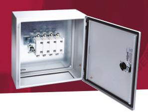
630A 4 pole switch disconnector in a metal enclosure to IP65. Enclosure has separate lock and reversible door for gland plate either top or bottom. The switch handle is padlockable and defeatable. All terminals are provided with shrouds. Earth studs are fitted and fixing brackets and earth straps are included
