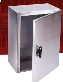
Wall mounting stainless steel enclosure with brushed finish. The polyurethane gasket keeps its profile over time to give a high degree of protection against water and dust. Door opens 125° and is reversible. Welded earth studs top and bottom. Fitted, galvanised backplate has return edges for extra rigidity
