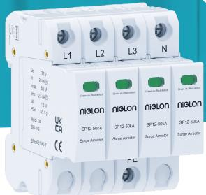
A four module three pole and neutral Type 1+2 combined lightning and surge arrestor with remote signal contact Suitable for use in incoming distribution panels where the risk of lightning strikes is high, particularly in buildings with a lightning protection system. Must be accompanied by downstream Type 2 surge protectors
