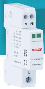
A compact single pole and neutral Type 2 combined lightning and surge arrestor with remote signal contact Suitable for use in distribution panels located downstream of Type 1 Surge arrestors, or distribution panels in areas with low exposure to lightning strikes
