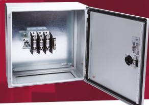
250A 3 pole and fixed neutral switch fuse in a larger metal enclosure to IP65. Enclosure has separate lock and reversible door for gland plate either top or bottom. The switch handle is padlockable and defeatable. The switch fuse accepts BS88 fuse links. All terminals are provided with shrouds. Earth studs are fitted and fixing brackets and earth straps are included.
