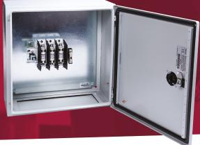
400A 3 pole switch fuse in a metal enclosure to IP65. Enclosure has separate lock and reversible door for gland plate either top or bottom. The switch handle is padlockable and defeatable. The switch fuse accepts BS88 fuse links. All terminals are provided with shrouds. Earth studs are fitted and fixing brackets and earth straps are included
