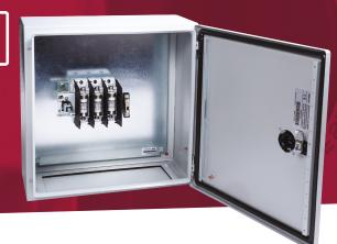
630A 3 pole switch fuse in a metal enclosure to IP66. Enclosure has separate lock and reversible door for gland plate either top or bottom. The switch handle is padlockable and defeatable. The switch fuse accepts BS88 fuse links. All terminals are provided with shrouds. Earth studs are fitted and fixing brackets and earth straps are included
