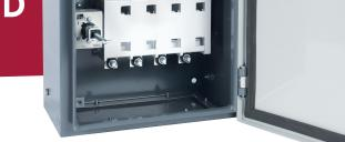
100A 4 pole switch disconnector in a compact metal enclosure to IP54. The switch handle is padlockable and defeatable. Earth studs are fitted.
