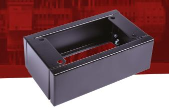
Plinths consist of 4 corner pieces, in 2mm steel, and 4 panels in 1.5mm steel, 2 depth profiles and 2 width profiles. All panels have return edges for added strength. Fixing bolts and accessories are included
