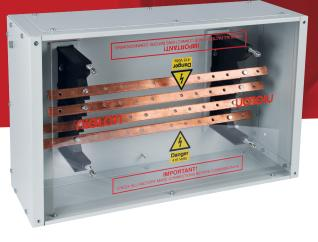
Fully rated and certified busbar chamber in steel enclosure with top and bottom blank gland plates and removeable side panels. Panels fixed with key hole slots. Single copper busbars have M6.5 holes at 50mm spacing for cable lug connection. Intended for use with the Niglon range of switch isolators and switchfuses
