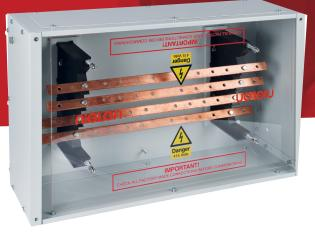
Fully rated and certified busbar chamber in steel enclosure with top and bottom blank gland plates and removeable side panels. Panels fixed with key hole slots. Single copper busbars have M6.5 holes at 50mm spacing for cable lug connection. Intended for use with the Niglon range of switch isolators and switchfuses
