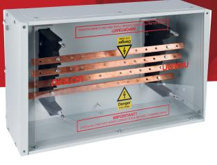
Fully rated and certified busbar chamber in steel enclosure with top and bottom blank gland plates and removeable side panels. Panels fixed with key hole slots. Single copper busbars have M6.5 holes at 50mm spacing for cable lug connection. Supplied in two sections with a joining kit for easy installation. Intended for use with the Niglon range of switch isolators and switchfuses
