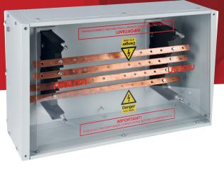
Fully rated and certified busbar chamber in steel enclosure with top and bottom blank gland plates and removeable side panels. Panels fixed with key hole slots. Single copper busbars have M10.5 holes at 50mm spacing for cable lug connection. Intended for use with the Niglon range of switch isolators and switchfuses
