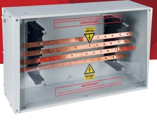
Fully rated and certified busbar chamber in steel enclosure with top and bottom blank gland plates and removeable side panels. Panels fixed with key hole slots. Single copper busbars have M10.5 holes at 50mm spacing for cable lug connection. Supplied in two sections with a joining kit for easy installation. Intended for use with the Niglon range of switch isolators and switchfuses
