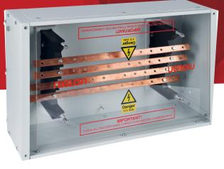
Fully rated and certified busbar chamber in steel enclosure with top and bottom blank gland plates and removeable side panels. Panels fixed with key hole slots. Single copper busbars have M10.5 holes at 50mm spacing for cable lug connection. Supplied in three sections with a joining kit for easy installation. Intended for use with the Niglon range of switch isolators and switchfuses
