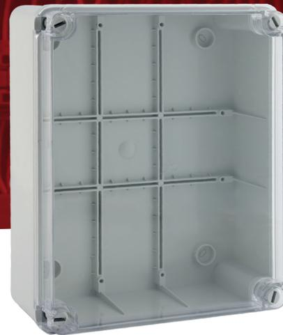
Multi purpose use junction box RAL7035 colour with transparent lid. High resistance to harsh weather conditions, corrosion and impact. Easily machinable with smooth sides and lid. Low profile lid is press fit and secured by 4 screws. Metal backplate available
