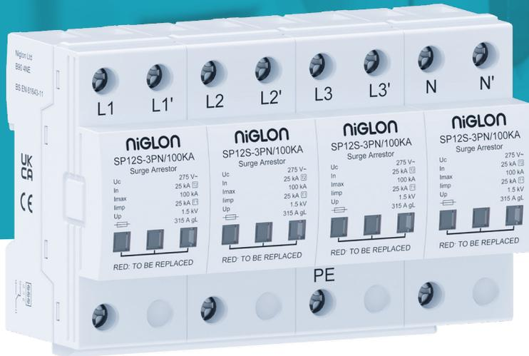
An eight module three pole and neutral Type 1+2 combined lightning and surge arrester with remote signal contact
