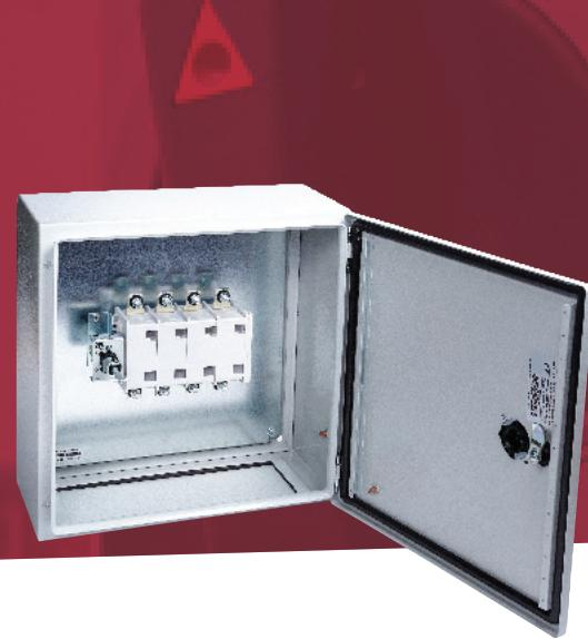
**250A 4 pole switch disconnector in a in a mild steel enclosure to IP54. Enclosure has separate lock. The switch handle is padlockable and defeatable. All terminals are provided with shrouds.**
